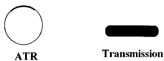
Figure 4. Two-dimensional drawing of the sampling volumes for the surface experiment using ATR mode, and the whole bead experiment using transmission mode. On the left, the cross-section of a bead in an ATR experiment is shown. The dark area shows the cross-section of the sampling volume. In the ATR mode, an ATR objective is in contact with a bead. Please note that although not shown in the figure, the bead may be slightly flattened when in contact with the ATR objective. The IR beam penetrates into the partial surface and is reflected with attenuated intensity. On the right, the cross-section of a flattened bead is shown. IR beam transmits the whole bead, and the sampling volume is the whole bead.
